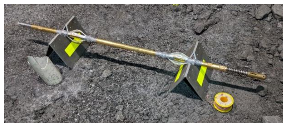
Centralizer blades mounted on running gear
